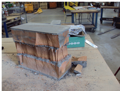
Fig. 2. A triplet after the compressive strength test
