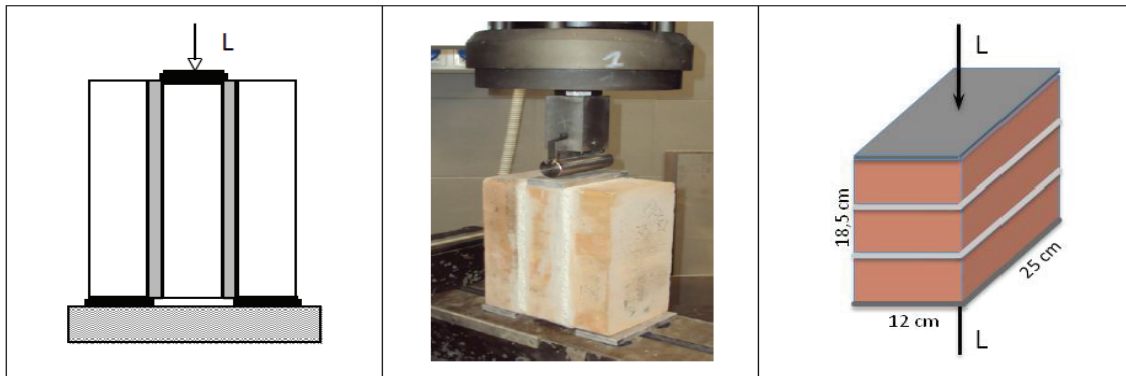
Fig. 1. Scheme of the shear and compressive test and a triplet during the testing
