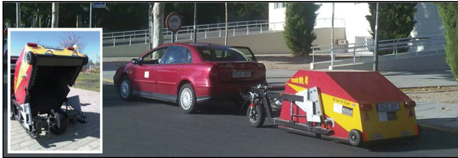
Fig. 3. Semi-anechoic chamber for the close proximity measurements
