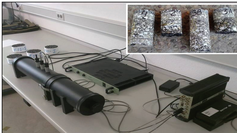
Fig. 5. Impedance tube and core samples from Crumb Rubber Modified Binder
