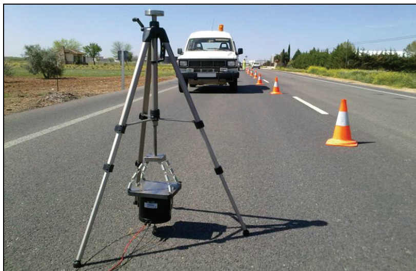
Fig. 4. Dynamic stiffness tests on the experimental test track with crumb rubber
