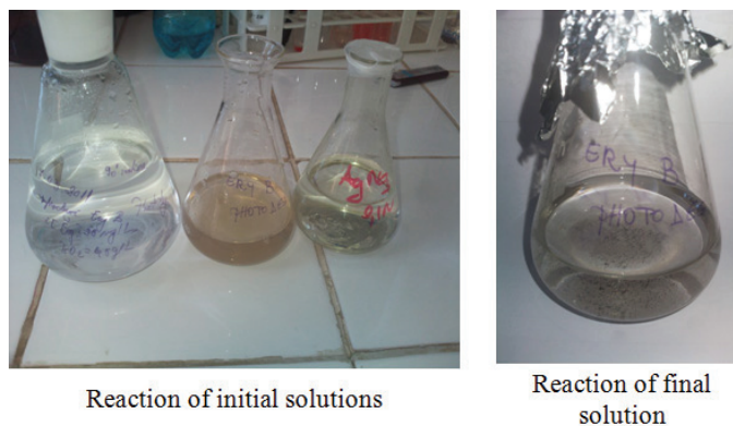
Fig. 3. The presence of I - in solution after Erythrosin B photodegradation
