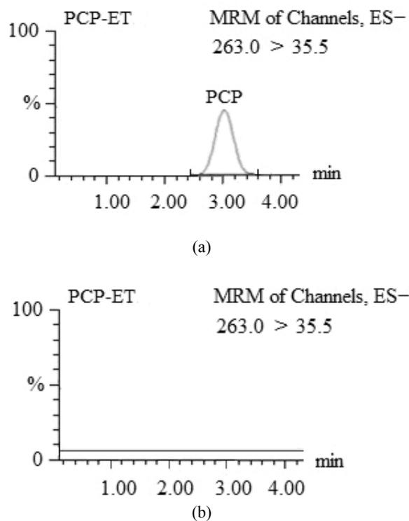
**Fig. 1.** Representative MRM chromatogram obtained from UHPLC/MS/MS analysis: (a) ultrapure water sample spiked with a standard solution of pentachlorophenol (concentration level IQL); (b) ultrapure water sample (blank)
